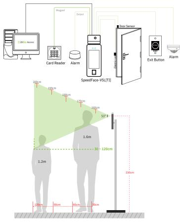
Recommended installation height: 150cm Temperature Measurement Distance: 30cm~120cm
